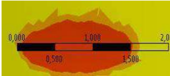
Fig. 4.12. Estimated area contact when loading on a roller 500 N
