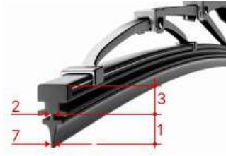
Fig. 1.2. R43 parameters of the cross-section of the wiper brush: 1 – 5 mm; 2 – 0.5 mm; 3 – 5 mm; 7 – 0.6 mm
