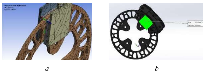
Fig. 1.32. Determination of pressure in the disc brake system: a) FEM model with load vector; b) determination of the brake pad area (SolidWorks environment)
