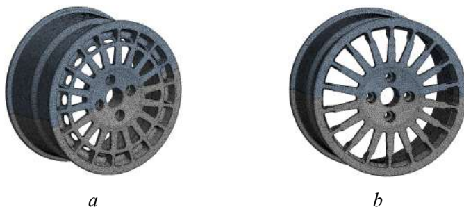
Fig. 1.45. FEA mesh of the 15-inch Lancia Delta HF Integrale rim: a) original design; b) without a ring
